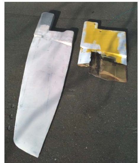
Comparison of the new and old daggerboard. Extensive CFD analysis reveals a reduction in drag of at least 0.045%.
